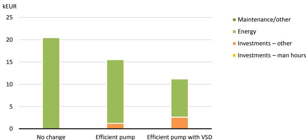
**Figure 10.** Life Cycle Cost for three different pump alternatives.
