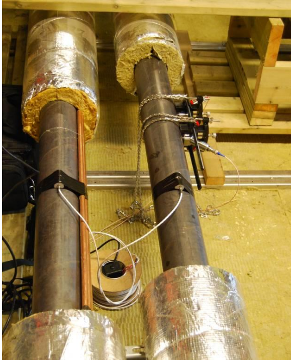
Figure 2. Example of mounting a mobile ultrasonic flow and heat meter.
